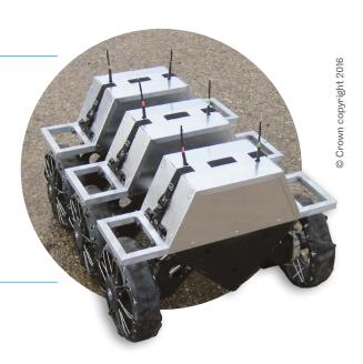
The DPG designed and manufactured a prototype modular explosion resistant vehicle (MERV) and sensor platform. The vehicle's key features include replaceable modules with an armour steel 'v' shaped outer hull designed to direct a blast away from the drive and control systems, secondary armour comprising 3D printed lattice structures and suspended systems trays within the hull assembly, designed to reduce transferred shock loadings from an explosive charge.
