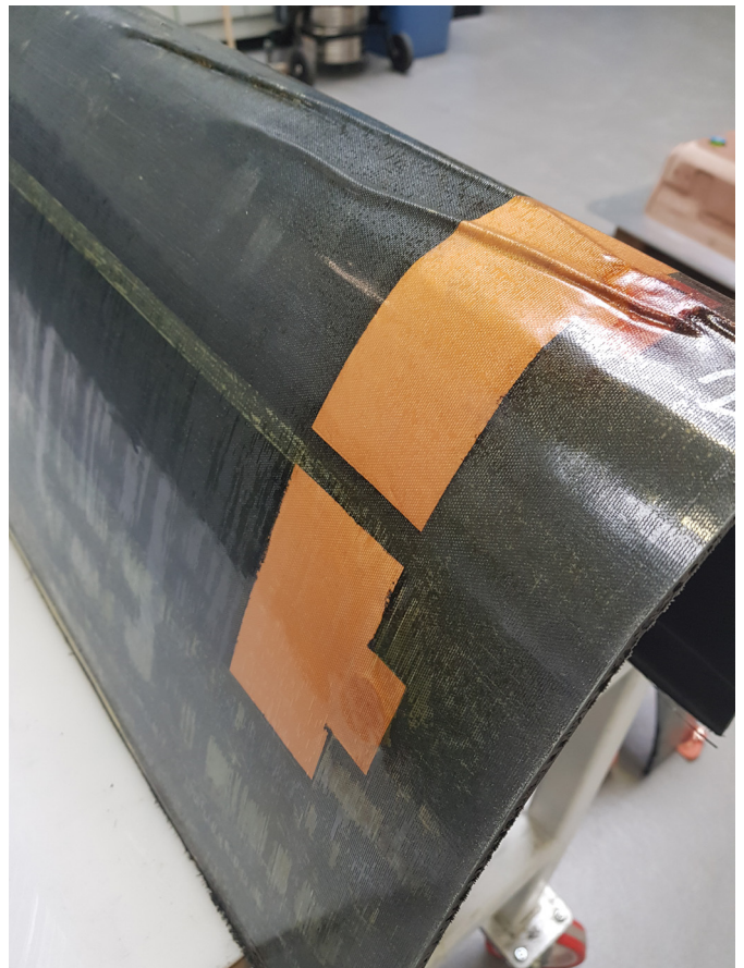
Final component showing the copper electrodes and unidirectional carbon fibre heaters below the glass fibre surface.
