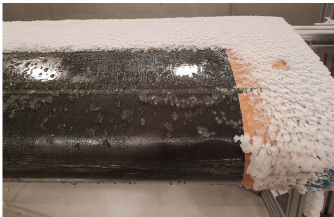
The demonstrator after the anti-icing testing had been completed, showing the difference between where the anti-icing had occurred and where there had been no heaters.
