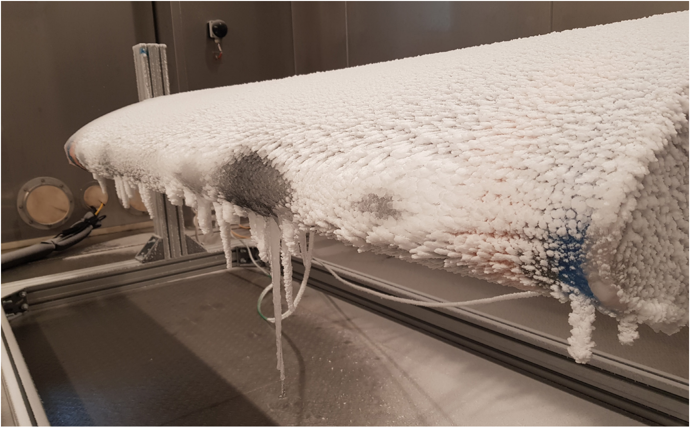
The final demonstrator in a climatic chamber, after being coated in ice at -15 °C, ready for the anti-icing test.
