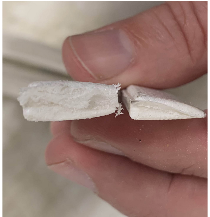
The process was developed to form fine foam geometry without spring-back. The increase in foam density also makes the thin sections more robust.
