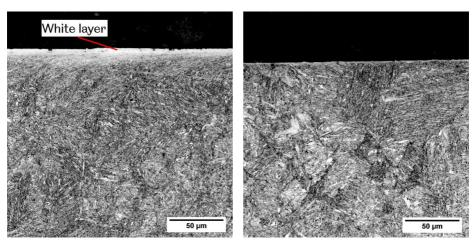
Left: Bad machined surface, created through turning using heavily worn inserts. Right: Conventional machined surface.
