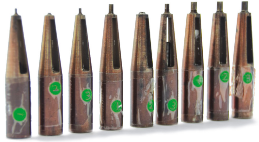
Testing samples to determine achievable torque for each size.
