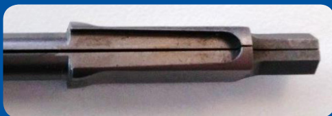
EDM machined slot down proportion of driver part.
