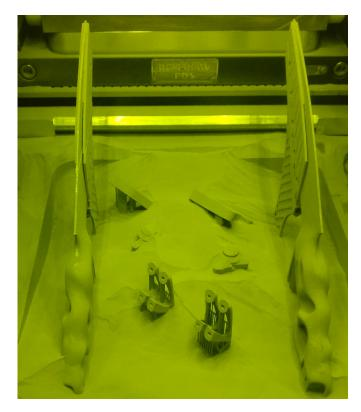
Above shows the knives during the additive manufacturing process and below the end result, complete with the novel support structures and thermal shrouding.
