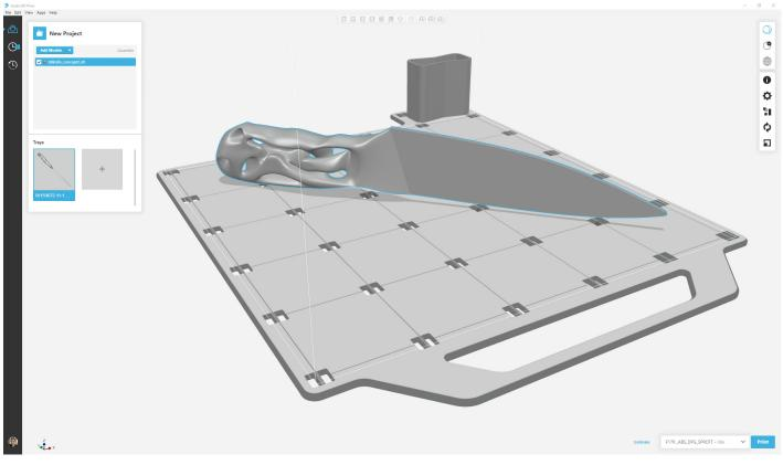
A GrabCAD print setup up of a concept knife model. At this stage the build orientation, supports and scan strategy is defined. Once the correct parameters are determined the knife is sliced and sent to a Fused Deposition Modelling (FDM) machine to be printed in polymer. Once 3D printed, this allows the designer to visualise the end concept cost effectively before moving onto metallic prototyping.
